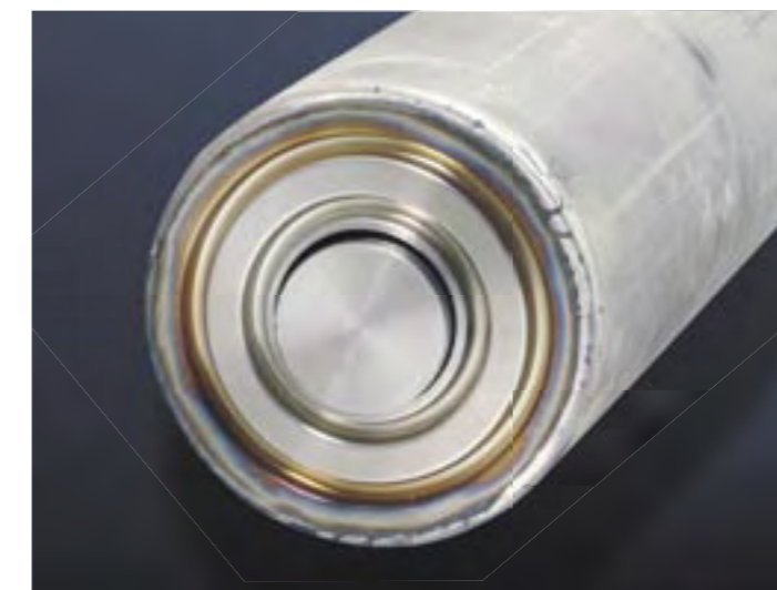
The tip of push plate inside the cooling protection jacket
