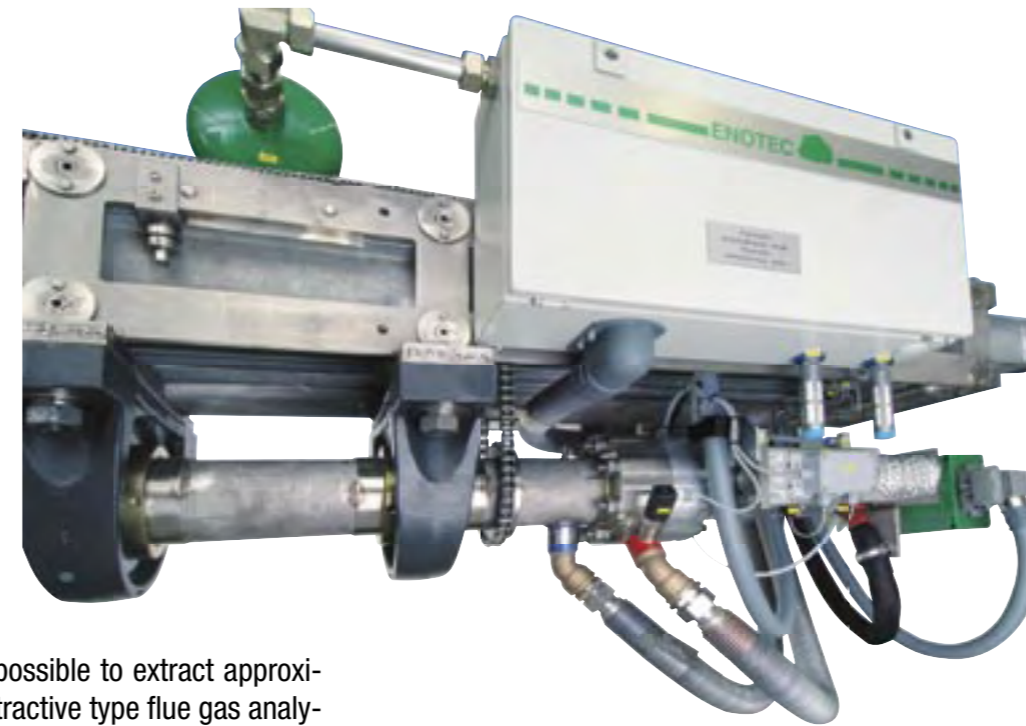
The CEMTEC®-terminal box with the pneumatic devices of the probe
